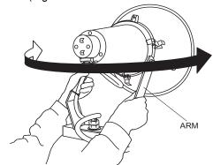
Figure 16. Adjusting Direction of Individual Lamp
